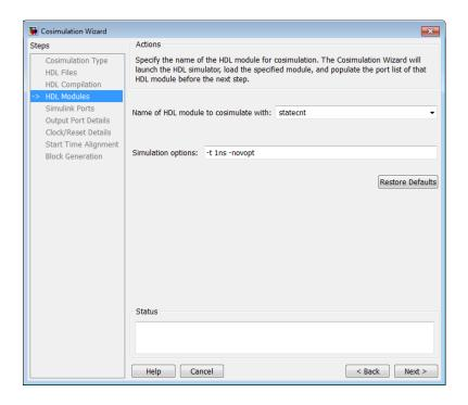
In the HDL Module Selection pane, provide the name of the HDL module to be used in cosimulation.
