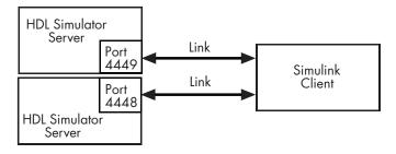
When you link the HDL simulator with a Simulink application, the simulator functions as the server. Using the HDL Verifier communications interface, an HDL Cosimulation block cosimulates a hardware component by applying input signals to and reading output signals from an HDL model under simulation in the HDL simulator.
