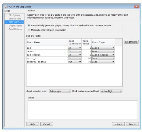
Step 5: Verify DUT I/O Ports for FIL Block
