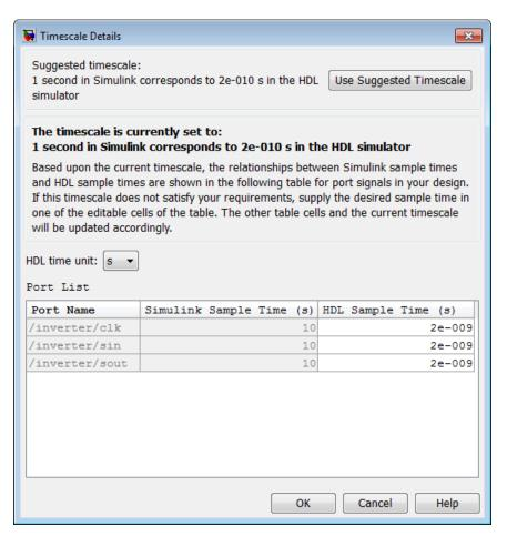
If you select Automatically determine timescale at start of simulation, you get the same dialog when the simulation starts in Simulink. Make the same adjustments at that time, if applicable, that you would if you clicked **Determine Timescale Now** when you were configuring the block.
