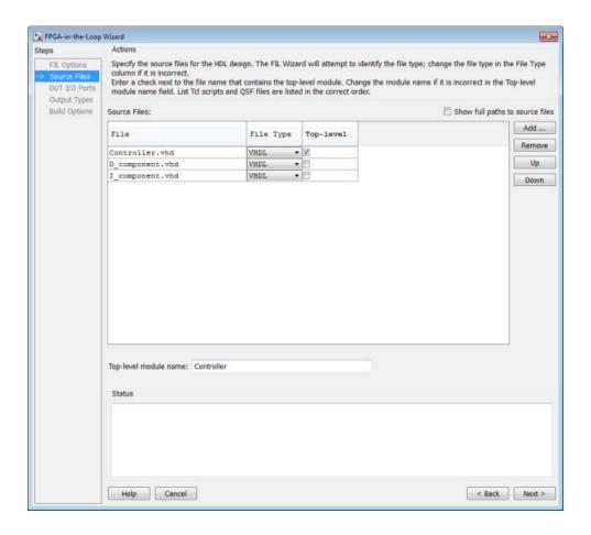
The FIL Wizard automatically fills the Top-level module name field with the name of the selected HDL file; in this case, **Controller**. In this example, the top-level module name matches the file name so that you do not need to change it. If the top-level module name and file name did not match, you would manually correct the top-level module name in this dialog.
