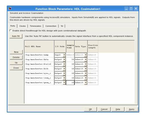
**Note** When you define an input port, make sure that only one source is set up to force input to that port. If multiple sources drive a signal, your Simulink model may produce unpredictable results.
