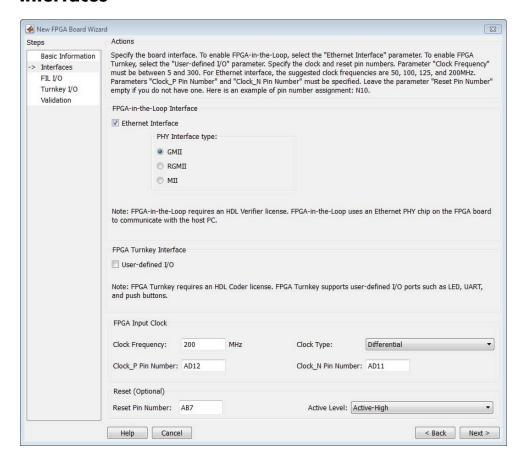
• FIL Interface: If you want to use this board with FIL, check Ethernet Interface. Specify the PHY Interface type (found in the board specification file).
