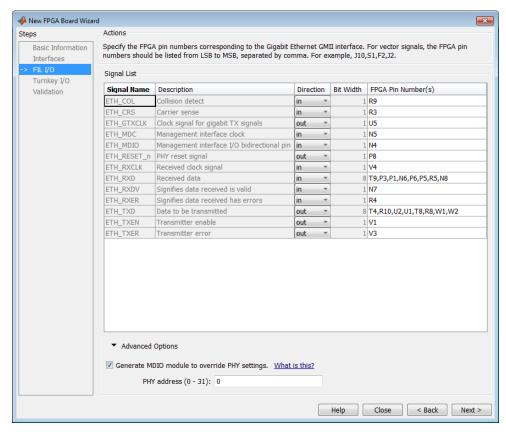
**Signal List**: You must provide all the FPGA pin numbers for the specified signals. You can find this information in the board specification file. For vector signals, list all pin numbers on the same line, separated by commas.
