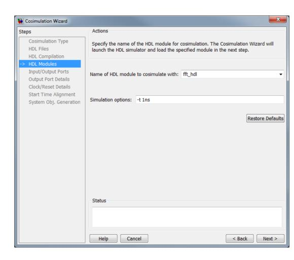
c. Click Next. The Cosimulation Wizard launches the HDL simulator in the background console using the specified HDL module and simulation options. If the wizard launches the HDL simulator successfully, the wizard populates the input and output ports on the Verilog model fft\_hdl and displays them in the next step.
