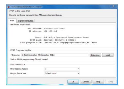
If your board is connected to the host computer through the JTAG cable properly, a message window displays to indicate that the FPGA programming file is loaded successfully. Click **OK** to dismiss this dialog.
