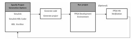
HDL Verifier packages generated files as a complete FPGA development environment project for use with Xilinx ISE.
