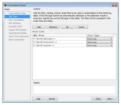
In the **HDL File** pane, specify the files to be used in creating the function or block.
