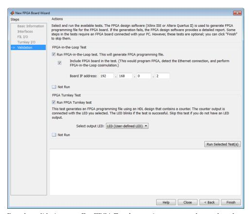
Run the validation test. For FPGA Turnkey testing, you must have a board attached. For FIL testing, the board is optional.
