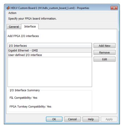
The Interface page describes the supported FPGA I/O Interfaces. Select any listed interface and click View to see the Signal List. If the board definition file has write permission, you can also Add New interface or Remove an interface.
