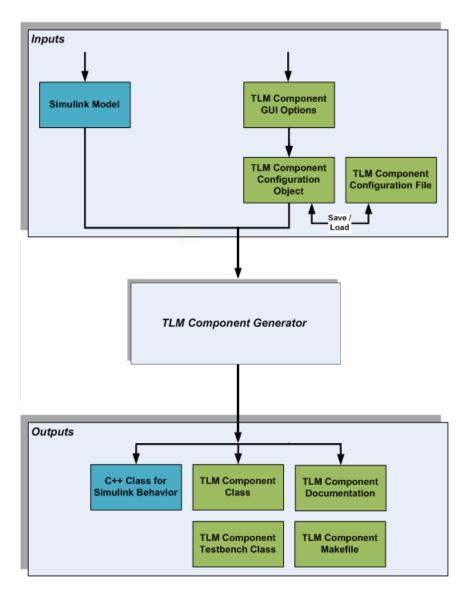
After code generation is complete, you can then use these generated files (outputs) to create the standalone TLM executable. See "Using the Generated TLM Component Files" on page 18-4.
