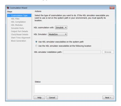
1 Select your HDL Cosimulation workflow in the field **HDL cosimulation** with: Simulink, MATLAB, or MATLAB System Object. This setting instructs the wizard to create a block, function template, or System object, respectively.
