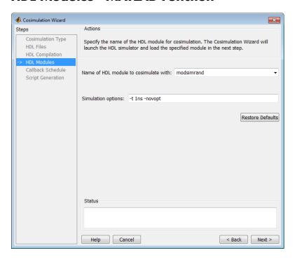
In the **HDL Module Selection** pane, provide the name of the HDL module to be used in cosimulation.
