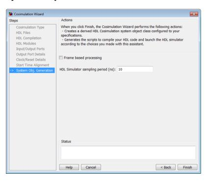
1 You can modify the HDL simulator sampling period before the wizard generates the System object. Enter the new value in the box labeled HDL Simulator sampling period (ns).
