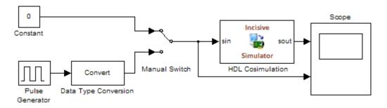
The model contains an HDL Cosimulation block (labeled HDL Cosimulation1) simulating an 8-bit inverter that is enabled by an explicit clock. The inverter has a single input and a single output. The following code excerpt lists the Verilog code for the inverter:
