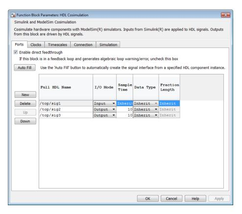
In this pane, you define the HDL signals of your design that you want to include in your Simulink block and set a sample time and data type for output ports. The parameters that you should specify on the **Ports** pane depend on the type of device the block is modeling as follows:
