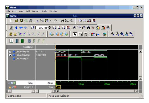
**5** In the Simulink Model, change **Constant value** to 2 and **Sample time** to 20 and start another simulation. This time, the value in the Display block changes to 253 and the ModelSim **wave** window appears as shown in the following figure.
