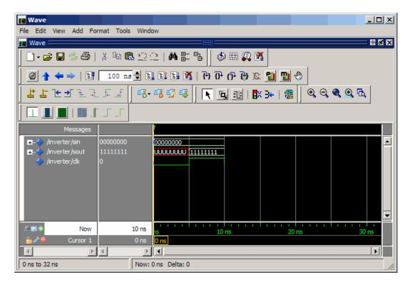
**4** In the Simulink model, change **Constant value** to 255, save the model, and start another simulation. The value in the Display block changes to 0 and the ModelSim wave window is updated as follows.
