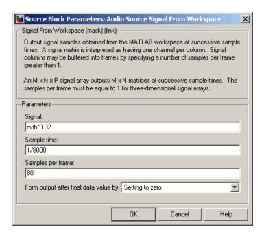
The sample rate and frame size of the input signal propagate throughout the model.
