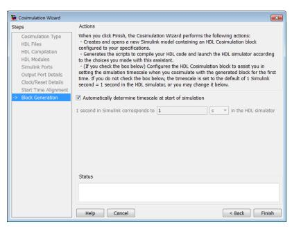
1 Specify if you want HDL Verifier to determine the timescale when you start the simulation by selecting **Automatically determine timescale** at start of simulation. If you prefer to determine the timescale yourself, leave this box unchecked and enter the timescale value in the text boxes below. The default is to automatically determine timescale.
