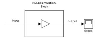
Without direct feedthrough applied, the HDL output has a one-sample delay compared with the Simulink reference signal, as shown in the following Scope window.
