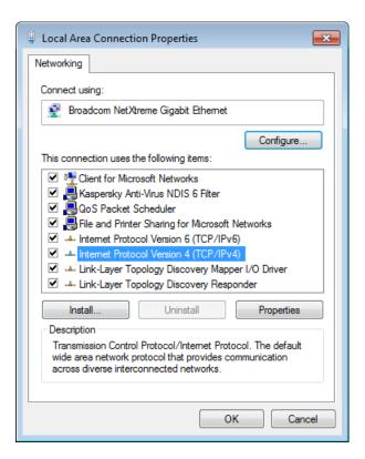
**4** Select **Use the following IP address** and set IP address to 192.168.0.1. If this address is in use by another computer on your network, change it to any available IP address on this subnet, such as 192.168.0.100. This value indicates your host computer address. Set the Subnet mask to 255.255.255.0.
