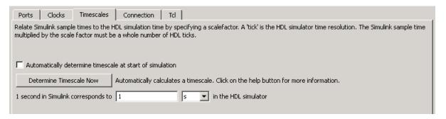
When you click **Determine Timescale Now**, HDL Verifier connects Simulink with the HDL simulator so that it can use the HDL simulator resolution to calculate the best timescale. You can accept the timescale
